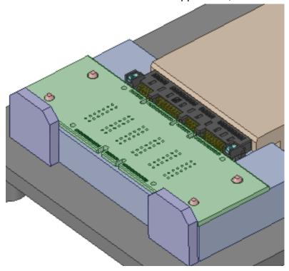
Step 3. Put connector assembled with PCB by wrench, then loosed the wrench;
